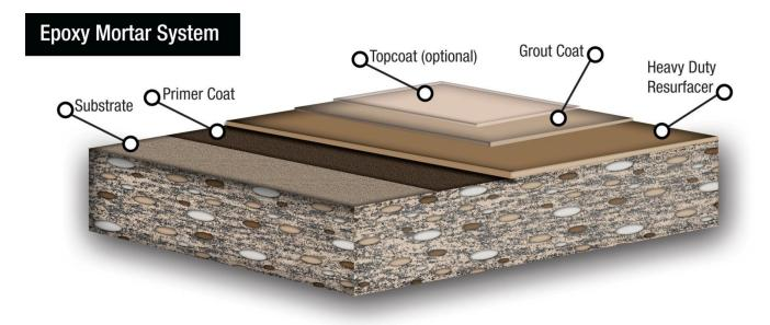
RS-21CF is a Heavy-Duty Epoxy Mortar Flooring System is a troweled, high strength concrete resurfacing material. It is used for low temperature environments (40F-60F) requiring an industrial grade floor or when a concrete floor has sustained damage requiring a 3/16" to 1/4" surface restoration.
